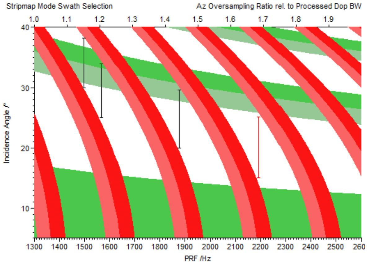
**Figure 3-13 : Swath Design 'Diamond Plot'**
