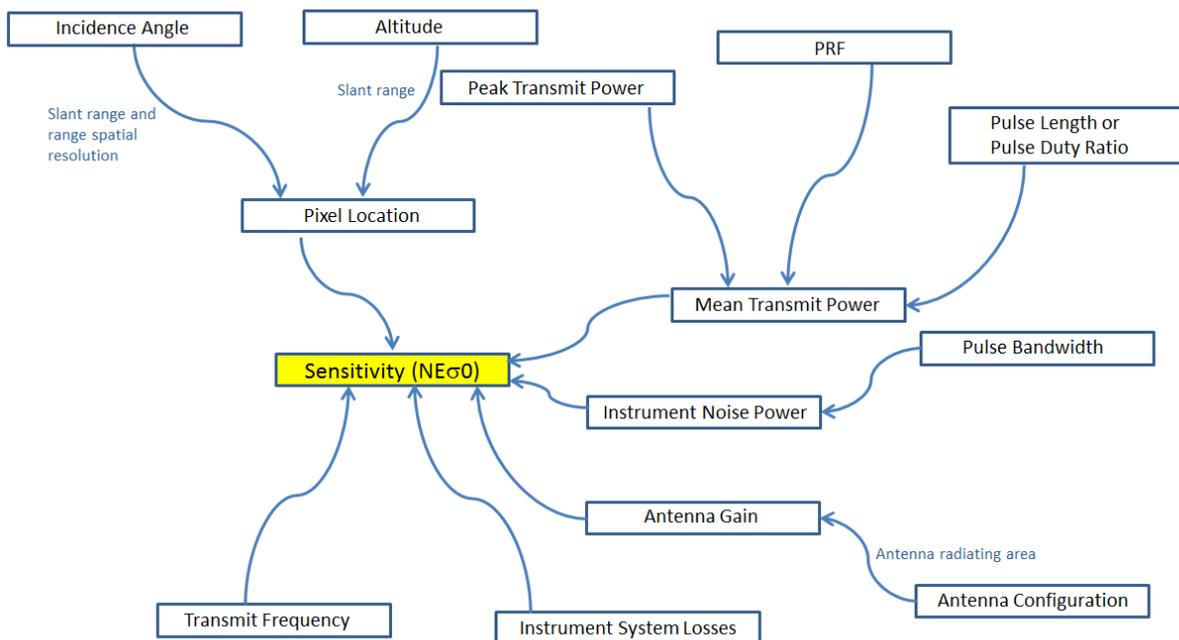
**Figure 3-6 : Radiometric Resolution Dependencies**
