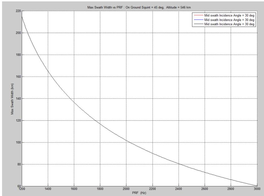
Figure 3-15 : Swath width v PRF for the Javelin configuration
