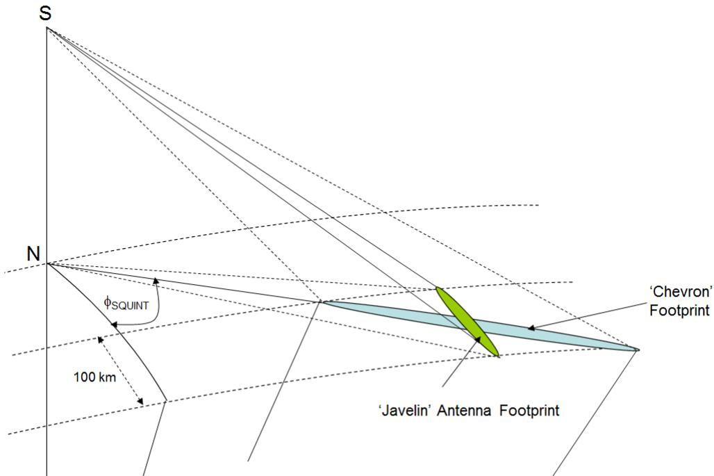
Figure 3-14 : Contrast between 'Javelin' and 'Chevron' beam positions.
