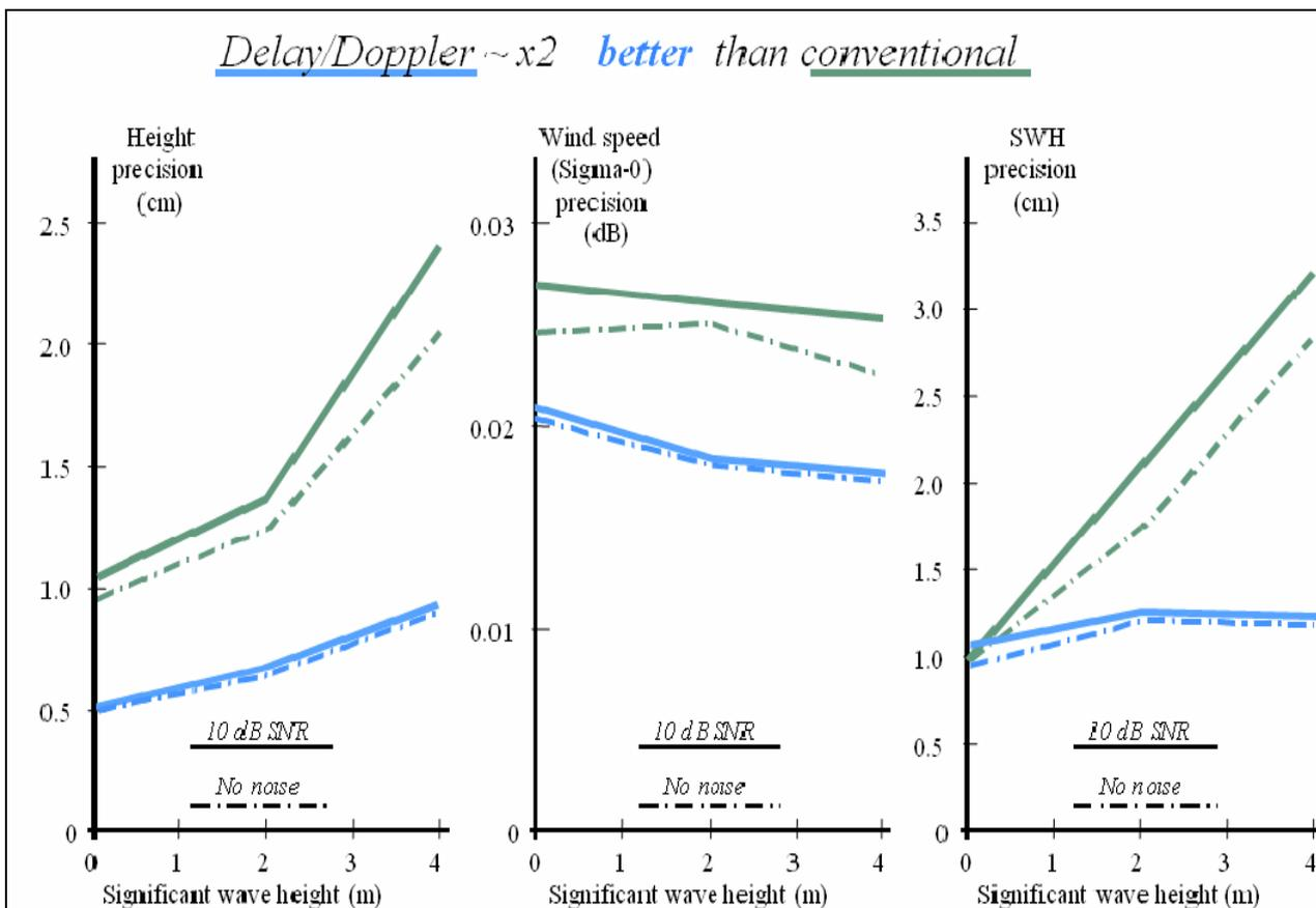
**Figure 1: Numerical estimates of the improved retrieval performance of Delay-Doppler Altimeters compared to conventional altimeters against SWH (Jensen & Raney, 1998)**
