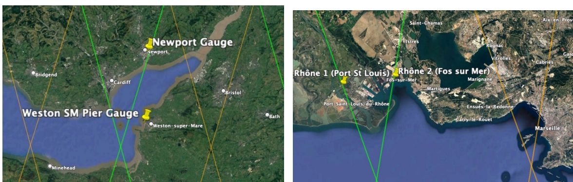
Figure 2.10 Locations of the vorteX.io micro-gauges. Left: on the Severn Estuary (UK), Right: on the River Rhône (France). The yellow pins show the locations of the gauges, the brown and green lines show the sub-satellite tracks of the Sentinel 3A and 3B satellite respectively.
