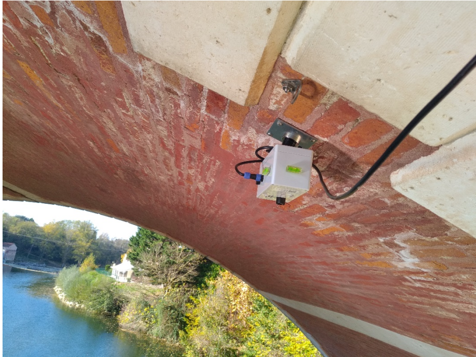
Figure 8: Illustration of a vorteX-io \mu VTX-1 installed under a bridge in the south of France
