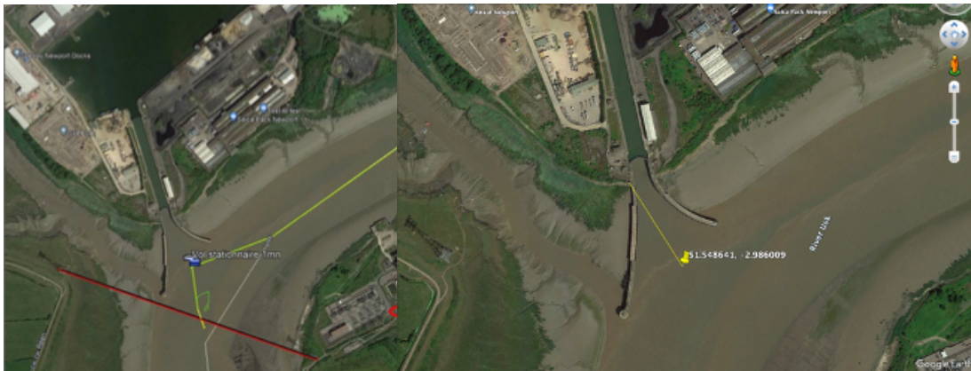
Figure A1 Left – drone flight trajectory and location of 1 minute hover at entrance to the Newport Harbour. Right - The NTSLF bubbler gauge is located on the western harbour pier (left) at the end of the yellow line, close to the lock gate. The NTSLF gauge is estimated to be 205m from the drone location.
