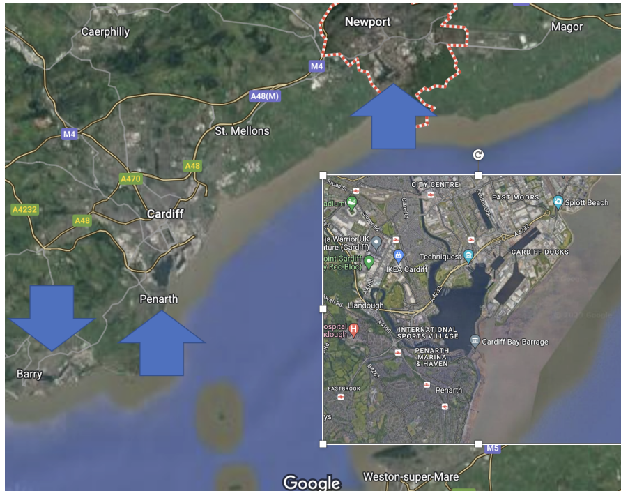
Figure 41. The expected causes for the snagging seen in the Sentinel-3B altimetry along track 254. The barracks at Newport, Cardiff, and Barry. The inserted picture is a zoom-in on Cardiff at low tides. The picture is from Google Earth.
