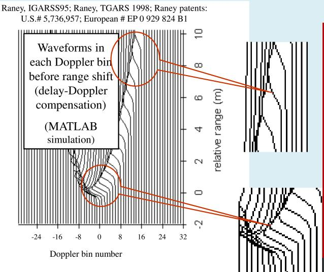
Waveform usefulness for determining range delay of the leading edge decreases as the square of the distance from nadir
