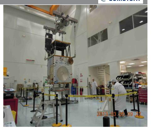
S3A alignment checks before starting with instrument integration
