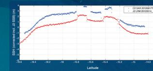
Good performances of Cryosat-2 SAR (red) data that continues to provide measurements across atolls in the Pacific, where conventional altimetry Jason-2 (blue) fails. Credits: NOC
