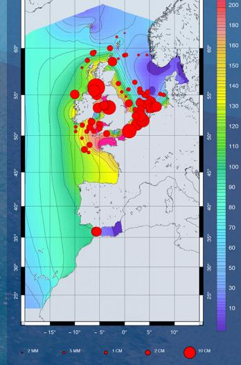
Amplitude of the M2 tidal wave from the COMAPI regional model (CNES project). The red dots superimposed are the vector differences between the model and tide gauge stations. The size of the dots is proportional to the misfit between the model and the observation. Credits: NOVELTIS
