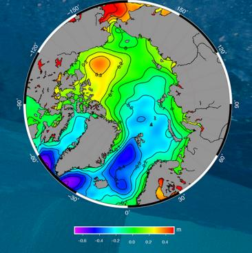
Cryosat-2 data provide important improvements to maps of Mean Dynamic Topography for the Arctic Ocean, and so support analysis of key ocean circulation features. Credits: DTU Space
