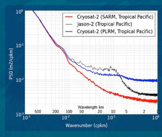
SAR mode (red) can resolve scales from 10-100km, not observable by conventional altimetry (Jason-2: Black, Cryosat-2 "Pseudo" LRM: blue) Credits: CNES/CLS
