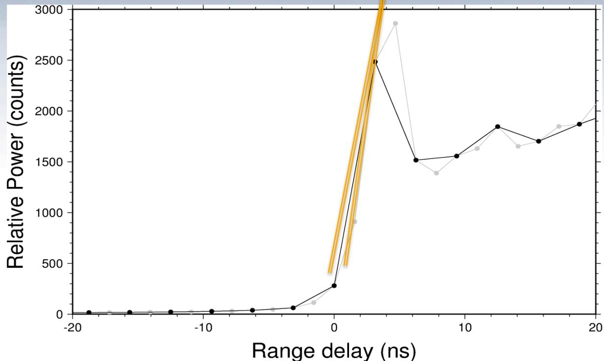
Increasing wave form samples from 128 to 256 using technique after Jensen (1999)
