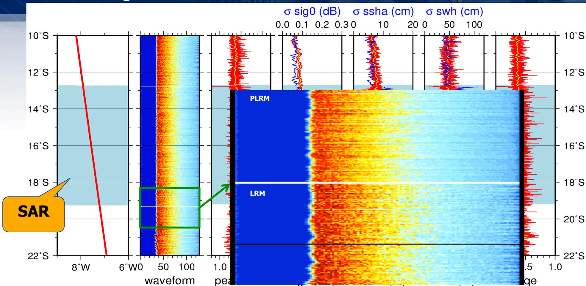
Waveform consistent between LRM and PLRM
