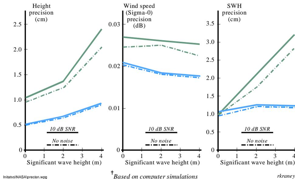
Figure 3. The simulated height precision, wind speed precision and SWH precision of 1 Hz observations derived with a DD instrument (bright blue curve) compared with a conventional satellite altimeter (green curve) (Jensen and Raney, 1998)
