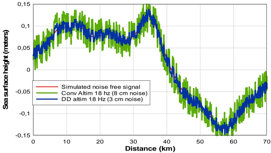
Figure 10. Simulation with the full 18 LRM DD observations and corresponding 18 Hz geodetic mission altimeter.
