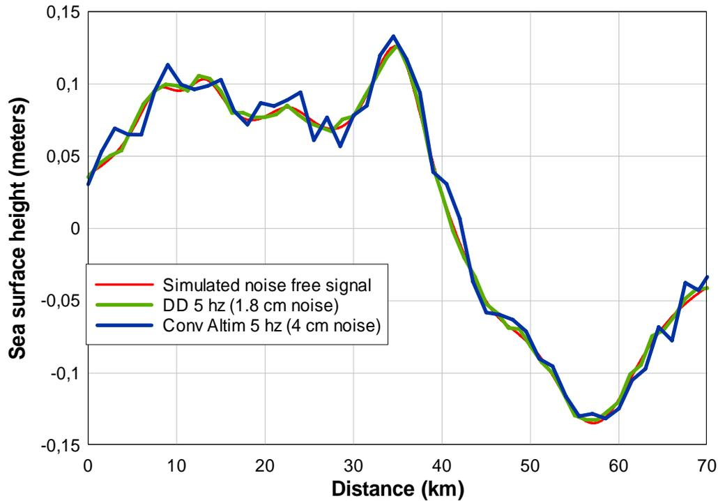
Figure 9. Simulation with 5 Hz DD observations and corresponding 5 Hz geodetic mission altimeter.
