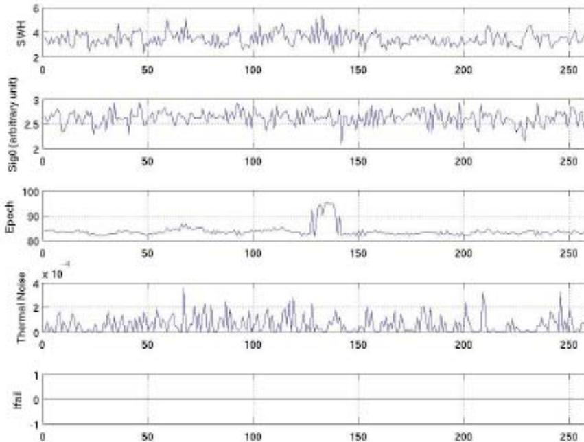
Figure 13. Output from the NOCS ocean re-tracker run on the CRYMPS LRM waveforms (scaled by 106) for scenario SFT1 (RV1). Top to bottom: retrieved SWH, Sigma0, epoch, thermal noise and retrieval quality flag). The bathymetric features shown in Figure 4 along the profile shown in Figure 5 are mapped.
