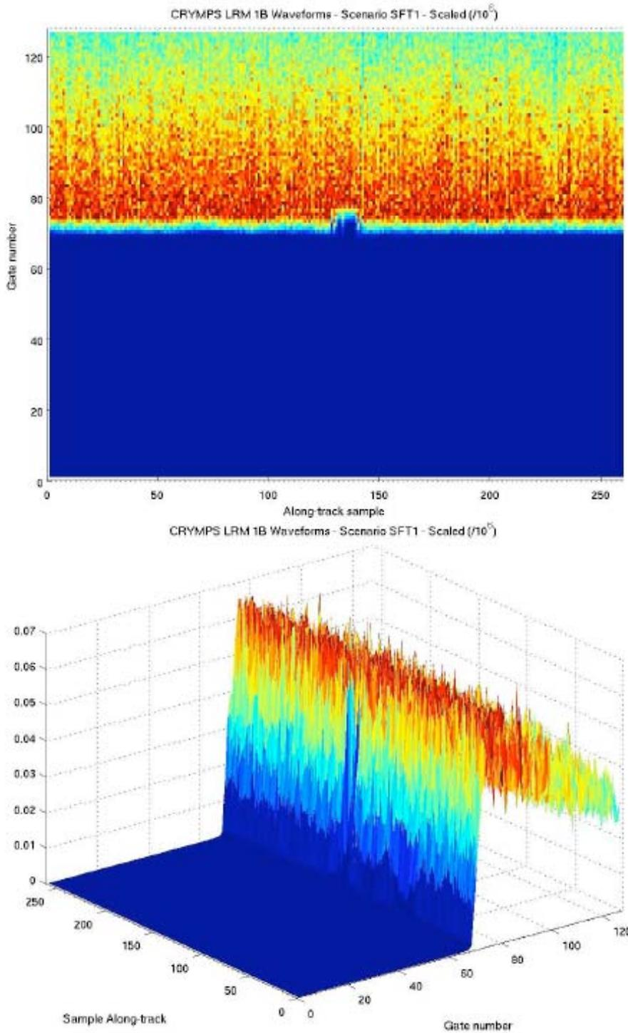
Figure 12 CRYMPS Low Resolution Mode waveforms for ocean with the bathymetric features shown in Figure 4 along the profile in Figure 5
