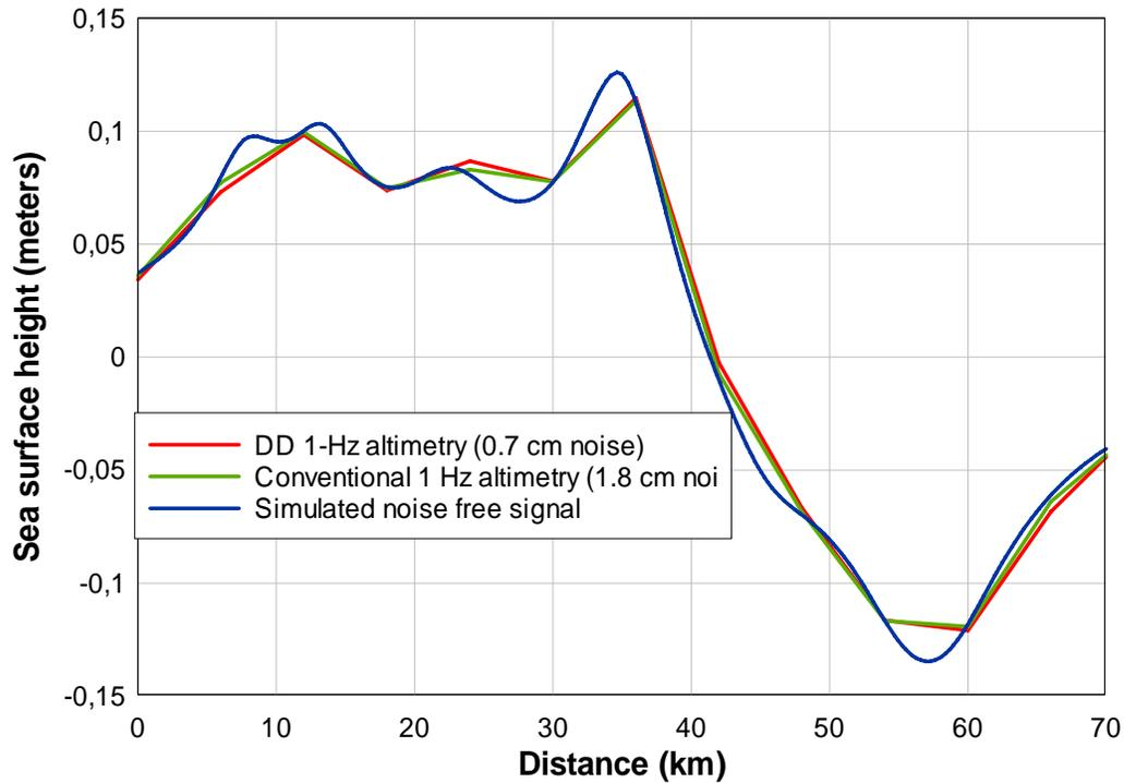
Figure 8. Simulation with 1Hz DD observations and corresponding 1 Hz geodetic mission altimeter. These conventional data are the typical data used to derive existing geophysical maps of the world's bathymetry.
